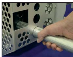
For situations many notches have to be made, Almi makes notching machines with a 2.2 kW electric motor.
